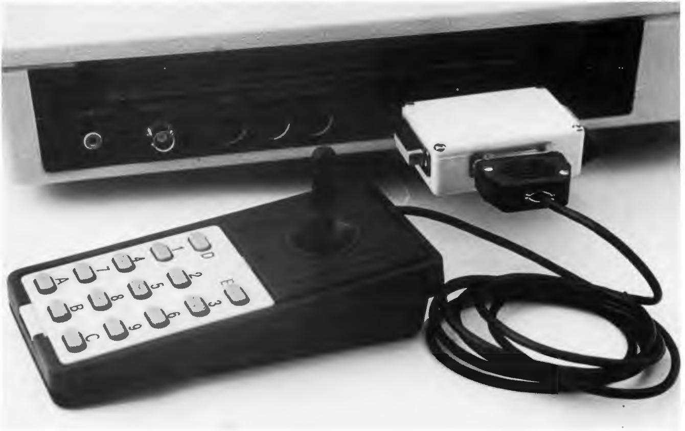
DELTA 14B HANDSET AND DELTA 14B/1 ADAPTOR BOX FOR THE BBC MICRO
